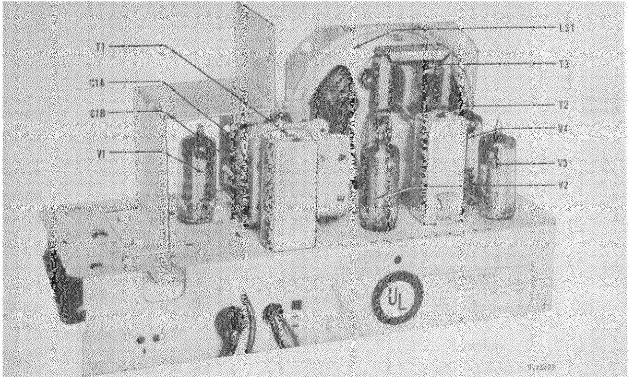
Fig. 5. Top View of Chassis Showing Component Location
