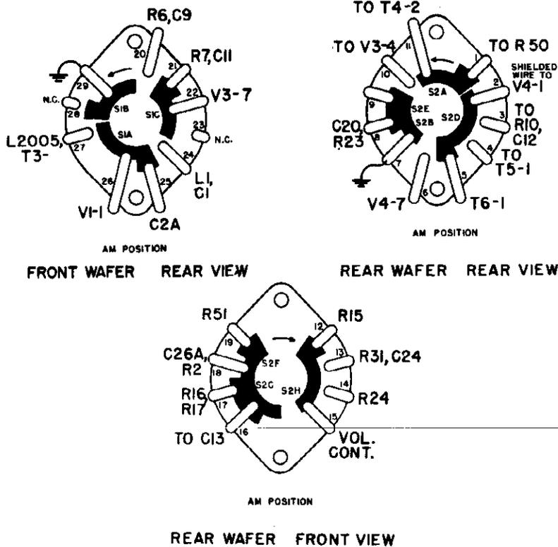
FIG. 7. SWITCH CONNECTIONS
