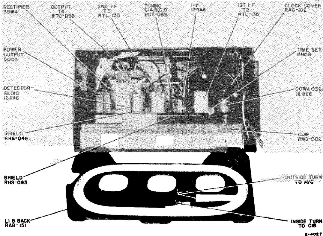
Fig. 1. Identification of Components, Model 514, Rear view
