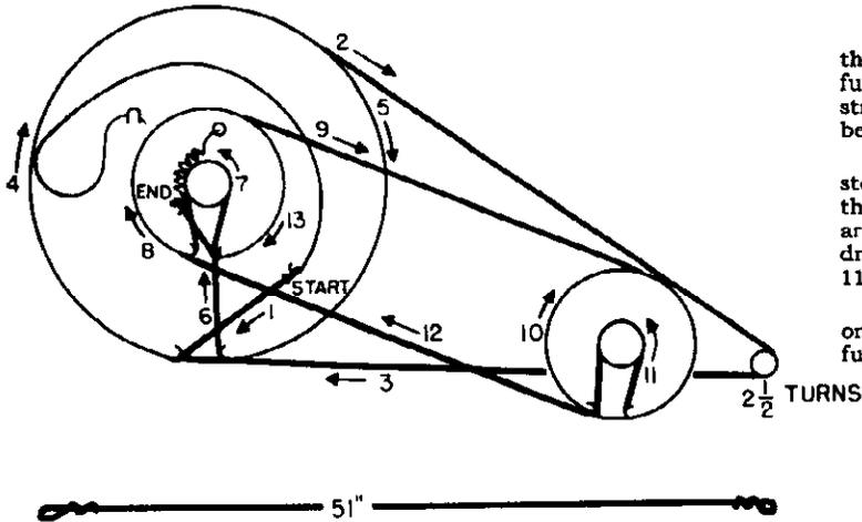
When stringing the dial cord both the A.M. and the F.M. tuning capacitor drums should be turned fully clockwise (minimum capacity). When the dial stringing is completed both tuning capacitors should be fully open or fully closed at the same time.
