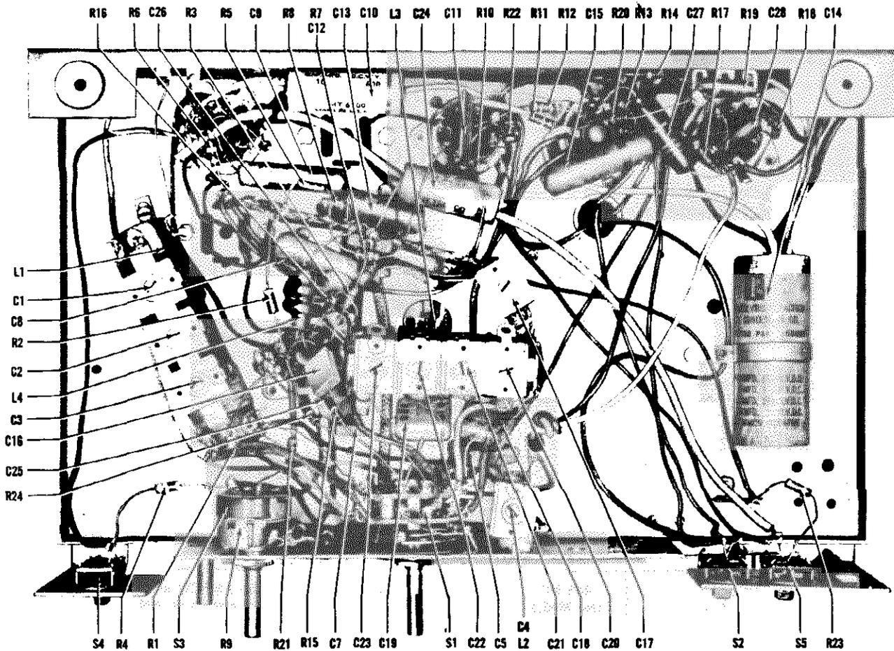
Fig. 6. Bottom View of Chassis Showing Component Location
