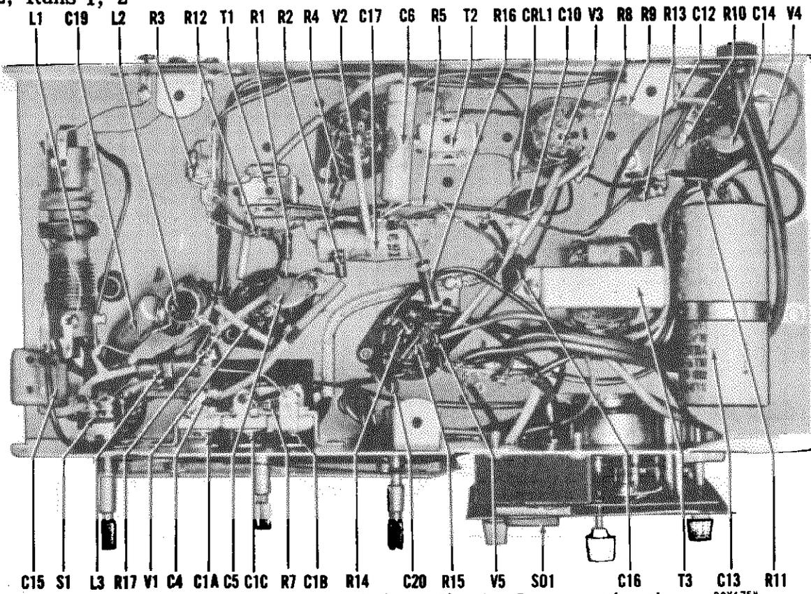
Fig. 11. Bottom View of Chassis Showing Component Location
