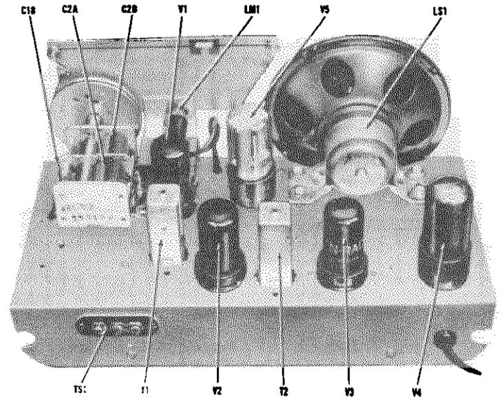
Fig. 4. Top View of Chassis Showing Component Location
