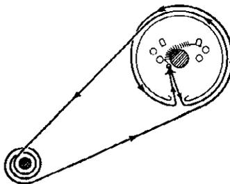
To string dial cord, turn the main drive drum to maximum counter-clockwise position and use following parts:
