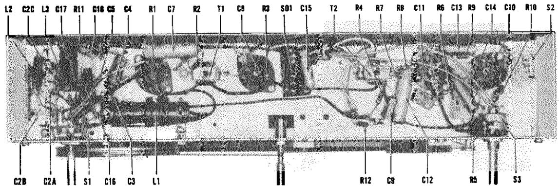
Fig. 6. Bottom View of Chassis Showing Component Location
