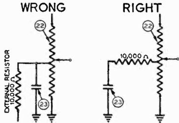
If a Philco 39-25 lacks high notes at low settings of the volume control, check to see how the bass-compensating condenser is connected. These partial schematics tell the story.
