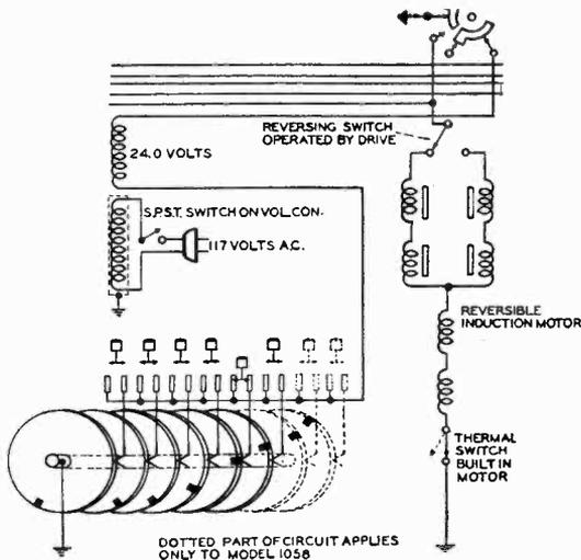
A new electric tuning system has been incorporated in later runs of Majestic models 11056, 11057, and 11058, the schematic being shown at the left. Note that the dotted portion of the drawing applies only to the last named model number.
