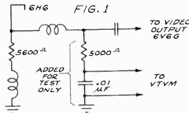
Leave generator connected to pin No. 4 of 2nd video i-f tube and connect the circuit shown in Fig. 1. A reading on the VTVM will prove continuity of video detector system. Be sure in this test signal-generator output is on maximum. Also that the VTVM will read a minimum of .25 volt. If not, this method cannot be used.
