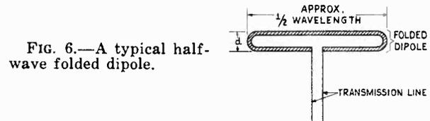
FIG. 6.—A typical half-wave folded dipole.
