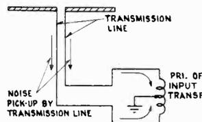
cancel each other. Hence, the total noise voltage induced in the secondary of the input transformer is effectively zero.
