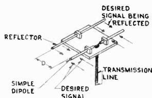
where a simple half-wave dipole is used, and placed behind this dipole and in the same plane of the dipole is the reflector element. This reflector conductor is usually of the same material as the dipole itself, and in practice it has been found that the reflector should be slightly longer than the length of the dipole used. The reflector should be placed on that side of the
