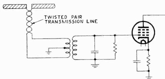
FIG. 5.—A simple impedance match for a half-wave antenna uses a twisted pair of transmission wires.
