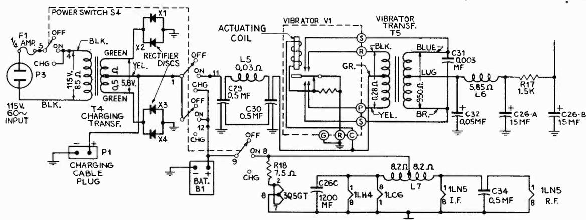
FIG. 6.—Power-supply and battery-charging circuits of the General Electric Model 250. The set is operated by a 2-volt storage battery, which can be charged from an automobile battery or a 115-volt a-c line.
