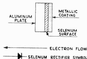
If the negative terminal of a power source is connected to the metallic coating, the flow of
