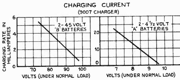
FIG. 4.—Graphs showing how the charging current of the batteries falls as they approach a charged condition.
