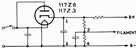
FIG. 13.—A typical rectifier circuit of an ac-dc receiver in which the internal tube resistance must be considered when replacing the tube with a selenium rectifier.
