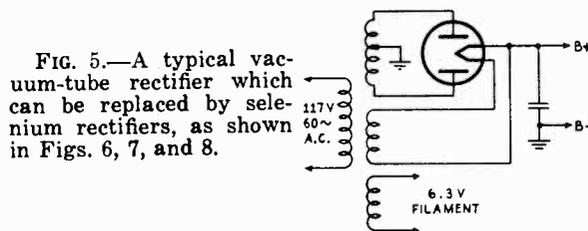
FIG. 5.—A typical vacuum-tube rectifier which can be replaced by selenium rectifiers, as shown in Figs. 6, 7, and 8.
