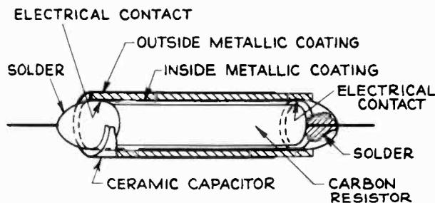
Fig. 5.—Detailed isometric cross-section of the R34-C48 unit.
