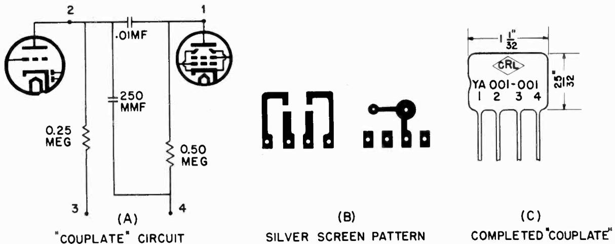
Fig. 14.—Schematic representation, silver screen pattern, and completed printed circuit for a coupling circuit are shown in parts (A), (B), and (C), respectively.
