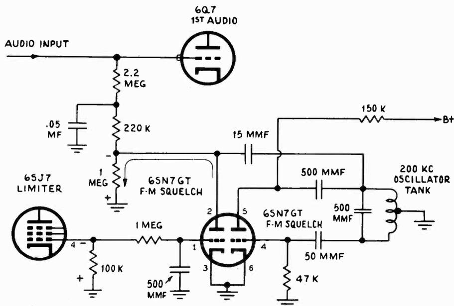
to see how it eliminates noise output from the receiver when tuning between f-m stations.
