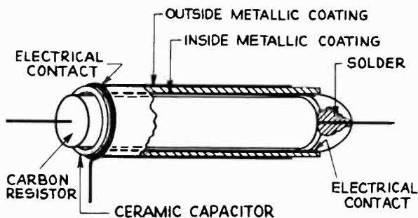
Fig. 3.—Enlarged isometric cross-section of the *R36-C52* unit.
