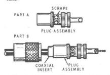
8. Solder the plug assembly to the shield wires through each of the four holes. Be sure you do not get solder on the threads. NOTE: You will need plenty of heat to do this properly. Then solder the inner wire (or wires) to the plug assembly and cut off any excess wire end.
