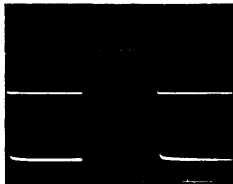
TOP TRACE: GATED OUTPUT 1V/DIV AND 50 \mu sec/DIV BOTTOM TRACE: VOLTAGE EXPANSION OF ABOVE SIGNAL—SHOWING NO RESIDUAL 1mV/DIV AND 50 \mu sec/DIV—AT LEAST 80 dB OF ISOLATION f_q = 100 kHz
