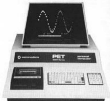
The self contained PET models 2001-4 and 8 come complete with TV screen, keyboard and built-in cassette deck as well as the computer circuitry. They are simply plugged into any 13 amp mains and no special knowledge is needed for running standard programs — over 200 of which are available on cassettes (please see separate software bulletins)
