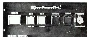
SERIES 3000 REMOTE CONTROL PANEL for record/playback unit with cue tones and fast forward option.
