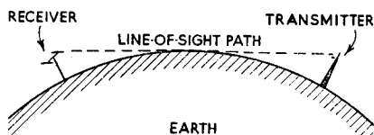
FIG. 8.2. The service area where a line-of-sight path exists between transmitter and receiver.
