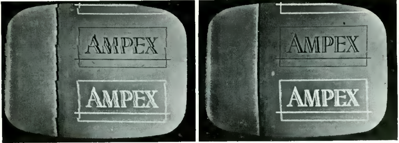
Fig. 5-24. The effect of Amtec on time-base errors.
