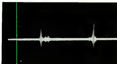
Fig. 6-4. Single-channel playback waveform with guide adjusted to barely contact tape.
