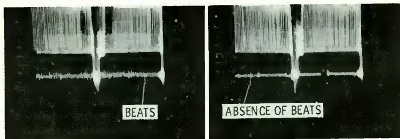
(B) External oscillator adjusted to zero beat with sync frequency.
