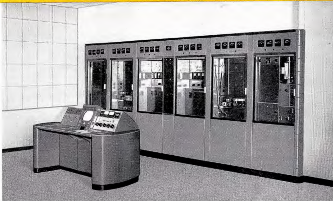
Typical transmitter installation showing the use of the TTC-1C Transmitter Control Console.
