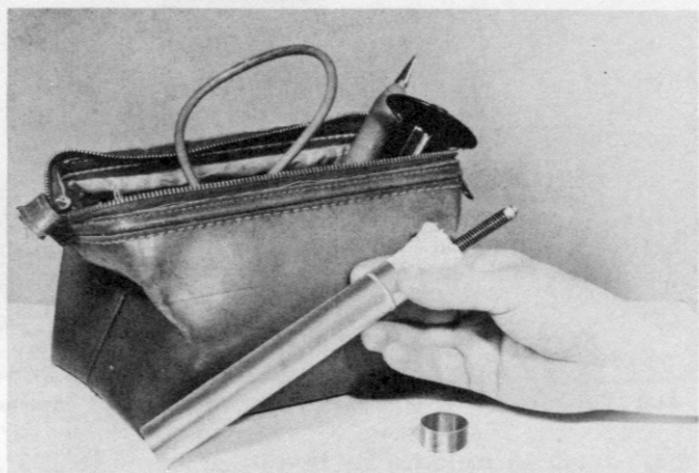
Fig. 619. The multiplier resistor in the probe is a barrier between you and the high voltage. Take care of it.
