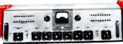
RCA Studio Console Type 76-C4. This flexible and easy-to-operate control unit performs all the audio amplifying, monitoring, and control functions of a TV station—large or small. Can be used for single- or two-studio operation, and for two transcription turntables.
