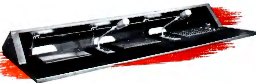
RCA Studio Console Type 76-C4. This flexible and easy-to-operate control unit performs all the audio amplifying, monitoring, and control functions of a TV station—large or small. Can be used for single- or two-studio operation, and for two transcription turntables.
