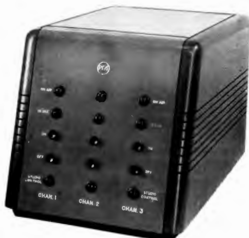
Studio Switching Console
