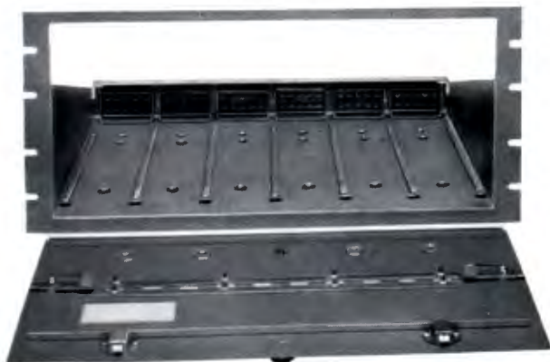
Panel removed showing guide bars and receptacles
