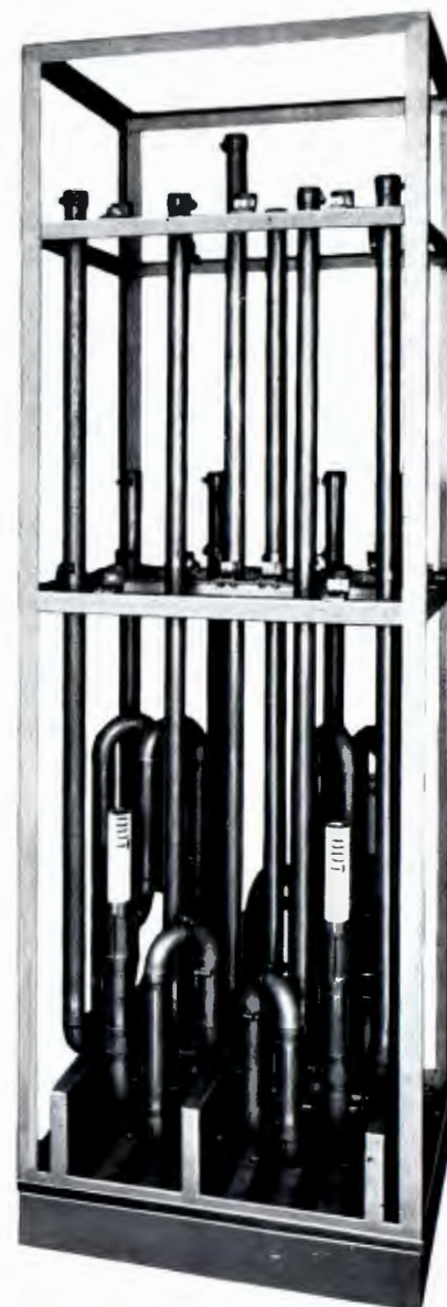
Triplexer with all covers removed to show system of tunable coaxial lines. Two output connections are made near the bottom, as shown. The two input lines are at the rear and are not visible.
