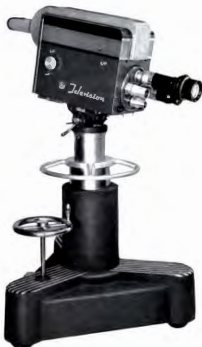
Studio type camera mounted on the pedestal.
