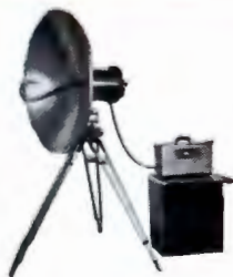
RCA Microwave Relay Transmitter TR-1A. Transmits the picture signals from field to studio (or from radio to transmitter). It includes a parabolic antenna with hook-shaped wave guide, built-in transmitter, and remote control unit. Matching receiver unit at the station picks up the microwave relay signal.
