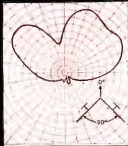
90° angle between dipoles 90° phasing between dipoles
