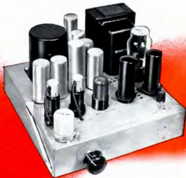
Monitoring Amplifier (Type BA-14A) —Designed for operation at microphone levels. High output of 12 watts is sufficient to drive several speakers or, in some applications, a recording head. Other uses include application as line amplifier for portable and mobile transmitters. High gain: 105 db. Low noise level: -20 db (with maximum gain); -40 db (with minimum gain). Low distortion: less than 3% at 12 watts. Frequency response: \pm 2 db, 30 to 15,000 cycles.
