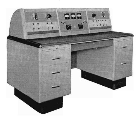
THE RCA MI-7237 Supervisory Control Console, illustrated in the accompanying photograph, has been styled and designed for use with the RCA Types 5-D, 5-DX and 10-D Broadcast Transmitters. All of the controls and indicating devices necessary for complete operation and observation of the transmitter are grouped conveniently and attractively in the sloping panels of the console turret top. This console also houses an RCA Type 82-A Monitoring Amplifier and an RCA Type 13-D Volume Indicator.
