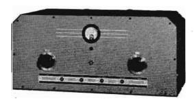
The ACT-20 Transmitter employs a three stage r-f circuit of unique design that simplifies adjustment when changing coils and crystals. The ACT-20 has a power output rating of 16 watts for 'phone and 20 watts C.W. throughout the operating range of 1715 to 30,000 KC. The r-f tube complement is as follows: RCA 807 crystal-controlled oscillator, RCA 802 buffer/doubler, RCA 807 power amplifier operating "Class C." The audio complement comprises an RCA 6F5 speech amplifier, RCA 6F6
