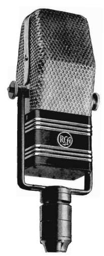
characteristics represent an almost equally attractive feature. The directional pattern is of the "figure eight" type, giving the microphone a bi-directional characteristic. This is a feature of considerable convenience as it provides a pickup configuration corresponding closely to average studio dimensions. Not only does it allow placing of artists on both sides of the microphone but it also, because of the dead sides, greatly reduces reflection from side walls.
