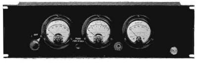
THE 15-B Meter Panel has been especially designed for use with the RCA Standard Line of speech input units. A patch cord is furnished with the 15-B for taking plate current readings and a two-way switch is provided for measuring the plate voltage from two sources. The A.C. meter is permanently connected in the circuit. The milliameter has a push-button providing two current ranges. When this meter panel is used with the 40-C and 41-B amplifiers, routine checking is easily accomplished, and in
