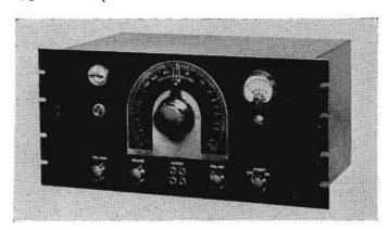
The Type 68-B Beat-Frequency Oscillator, used in conjunction with the Type 69-A Distortion Meter described on page 10, is ideal for making harmonic distortion measurements on broadcast transmitters. Another unit useful in this application is the Type 89-A Attenuator Panel, by means of which suitable attenuation can be introduced to feed the distortion meter and the equipment under test. This unit, described on page 11, will save considerable time in setting up equipment for measurement.
