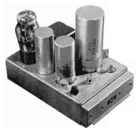
THE MI-4303 Power Supply is intended to furnish plate and filament voltages for a maximum of two Type 85-A Preamplifiers or 85-X Isolation Amplifiers or one 41-B Preamplifier. It contains a hum control potentiometer across the filament supply. A power switch and a ½ ampere glass fuse is provided. Three MI-4303 power supplies may be mounted on one 36-A or 36-B Panel.
