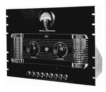
tions in the a-c line voltage. The front panel illuminated meter is connected to a 3-position switch so it may be used for (1) indicating plate currents, (2) indicating "db" of compression, or (3) indicating audio output level in db.
