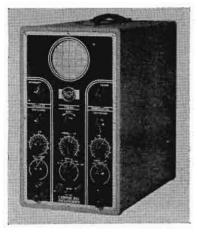
Description: An instrument of laboratory standards of performance, whose moderate size and weight make it at the same time conveniently portable for service use. It uses the RCA-906 3-Inch Cathode-Ray Tube giving a brilliant, clear pattern. An integral timing-axis oscillator provides saw-tooth potentials to the deflection plates for horizontal deflection of the cathode-
