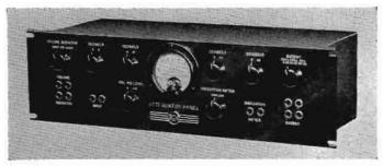
Applications: The Type 89-A Attenuator Panel greatly facilitates use of the Type 68-B and 69-A instruments by simplifying the work of setting up equipment for various measurements. It is particularly useful in broadcasting stations and laboratories because the improvement in operating convenience means a saving of much valuable time. It contains an excellent volume indicator, useful also for general measurement purposes.
