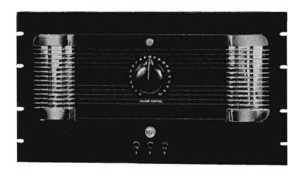
THE RCA 55-B is a bridging or line amplifier useful for isolating a program channel from an outgoing line. Where a single program is fed to several points, such as to a network, a local station and to a short wave transmitter, it is important to prevent any one of the lines from affecting the others. The 55-B has been designed for isolating lines but it is also valuable for other purposes where a gain of 45 db. is required.
