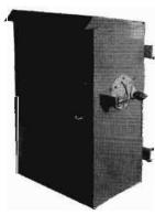
THE MI-7423, Type AZ-4293 Antenna Tuning Unit provides for terminating a transmission line, and matching the line of a broadcast transmitter to the antenna radiator. It is designed to match a transmission line having an impedance of 70 to 350 ohms, one side of which is grounded, to an antenna having a reactance of plus 200 ohms to minus 200 ohms and a resistance of from 20 to 200 ohms.
