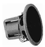
THE TYPES UZ-4209 and UZ-4309 Units are unmounted 8" high-fidelity loudspeakers especially designed for use with RCA Deluxe Speech Input Systems. They are particularly useful in control booths, and other locations where floor space is limited, in that they can be mounted on flat baffles and suspended from the ceiling or wall. Mounted in a large flat baffle, they have a uni-
