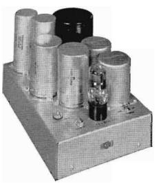
THE MI-11302 Power Supply has been designed to furnish plate and filament voltages to a maximum of ten Type 85-A Preamplifiers or 85-X Isolation Amplifiers. It will furnish plate voltage to 3 Type 41-C Preamplifiers or 9 Type 41-B Preamplifiers. It contains a hum control potentiometer across the filament supply and an output voltage regulating potentiometer. A power switch and a 1 ampere glass fuse is provided. Two MI-11302 power supplies may be mounted on one 36-A or 36-B Panel.
