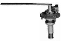
THE MI-4861 Tonearm Lift adds to the convenience of operating the 70-B turntables or the MI-4857 Lateral Kits with 70-A turntables. It is cam operated and permits lowering the pickup in any predetermined position. A minimum drop adjustment is provided which prevents the pickup point from striking the platter felt if it should run off the outer edge of the record-a valuable feature in safeguarding the diamond point.
