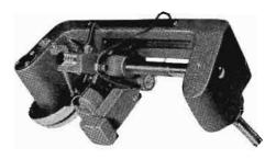
Float Stabilizer mounted on the type 72-B recording attachment
