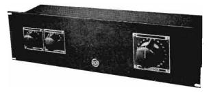
ONE of the four line equalizing units for use with RCA transmitter installations, the RCA 56-B is a rack mounting panel equipped with a variable ladder type pad in the output for controlling gain and with the network resistors variable from the panel. A repeat coil is included. This unit is desirable where equalization is likely to be varied or where one equalizer is not tied up permanently with a line.
